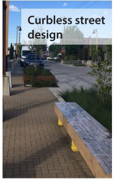
Curb ramps permit people using wheelchairs or pushing a stroller to cross more easily. Alternatively consider eliminating curbs altogether to allow unimpeded flow of pedestrians.
